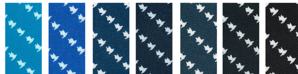
Turquoise Blue PGR 30 g/kg Brill. Blue P3R 30 g/kg Navy P2R 30 g/kg Navy Blue HF 30 g/kg Black PN 30 g/kg Black PGR 50 g/kg Black DG 50 g/kg
