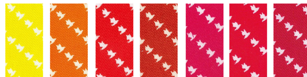
Yellow P6G 30 g/kg Golden Yellow P3R 30 g/kg Orange P2R 30 g/kg Orange P4R 30 g/kg Red P3B 30 g/kg Red P4BN 30 g/kg Red P6B 30 g/kg
